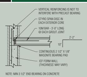
VERTICAL REINFORCING IS NOT TO INTERFERE WITH PRECAST BEARING
