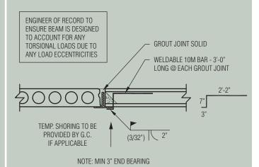
ST9 End to End Bearing — Back to Back Angles **ST10**
