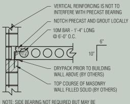
NOTE: SIDE BEARING NOT REQUIRED BUT MAY BE USED TO PROVIDE LATERAL SUPPORT TO WALLS
