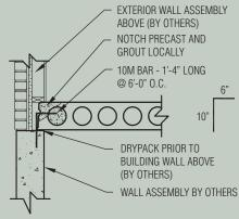
NOTE: SIDE BEARING NOT REQUIRED BUT MAY BE USED TO PROVIDE LATERAL SUPPORT TO WALLS
