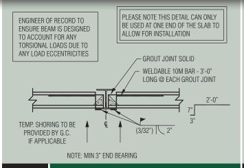
ENGINEER OF RECORD TO **ENSURE BEAM IS DESIGNED** TO ACCOUNT FOR ANY **GROUT JOINT SOLID** TORSIONAL LOADS DUE TO 1/2" STRAND - 4'-0" LONG ANY LOAD ECCENTRICITIES @ EACH GROUT JOINT TEMP. SHORING TO BE PROVIDED BY G.C. IF APPLICABLE NOTE: MIN 3" END BEARING
